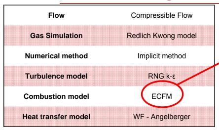
LFS submodel from detailed chemistry developed and implemented via UDF
