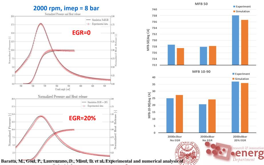
diluted combustion in a direct injection CNG engine featuring post- Euro-VI fuel consumption targets. Submitted to the SAE WCX 2018 Congress.
