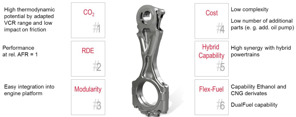
Fig. 2: Major requirements of VCR system in gasoline powertrains
