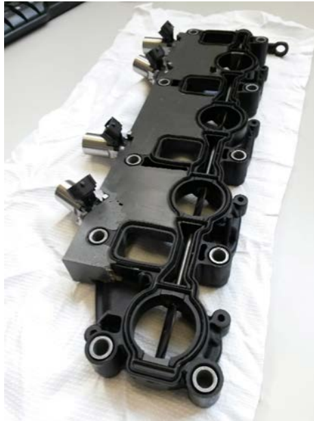
Figure 4: Four PFI gas injectors mounted on the swirl flap adapter of the original diesel engine
