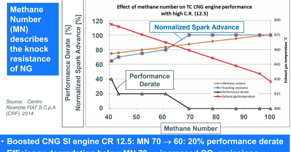
• Efficiency degradation below MN 70  $\rightarrow$  increased CO<sub>2</sub> emissions
